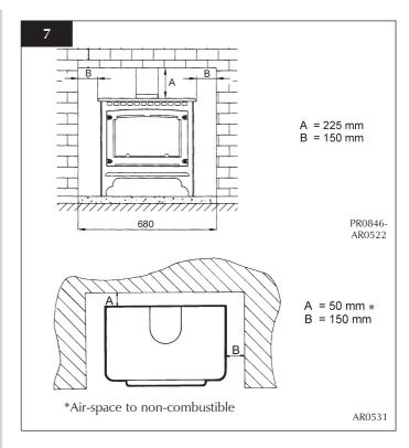
The above dimensions provide adequate clearance at the side and rear of the fire so that the controls can be reached.
